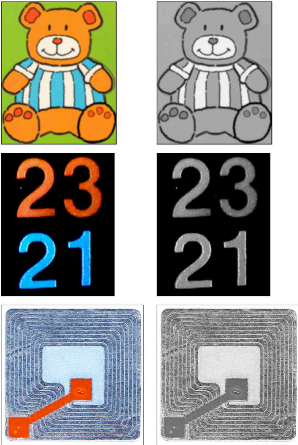
Situations in which intensity fails to provide satisfactory discrimination. (Top-left) Original image. [Child's ji-saw puzzle, printed card] (Top-right) Intensity. (Centre-left) Original image. [Thermo-chromic paint, used as thermometer] (Centre-right) Intensity. (Bottom-left) Original image [RFID] tag. (Bottom-right) Intensity.
