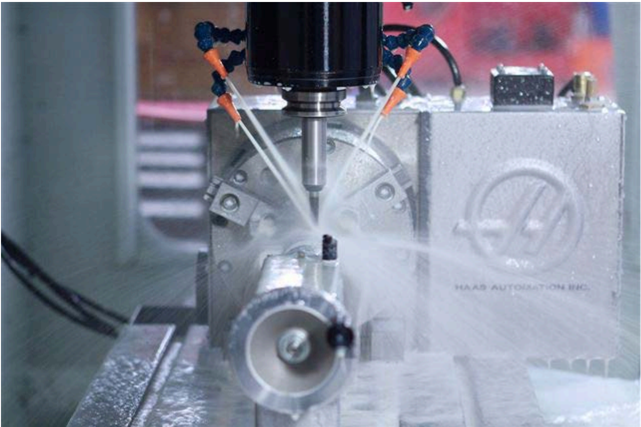
Figure 2.6 Factories are sometimes very dirty places! Placing an unprotected camera and lights close to a machine tool such as this lathe would be foolish. Apart from the obvious cloud of cutting fluid, numerous tiny droplets are created in the atmosphere and can quickly contaminate optical surfaces, degrading image quality.
