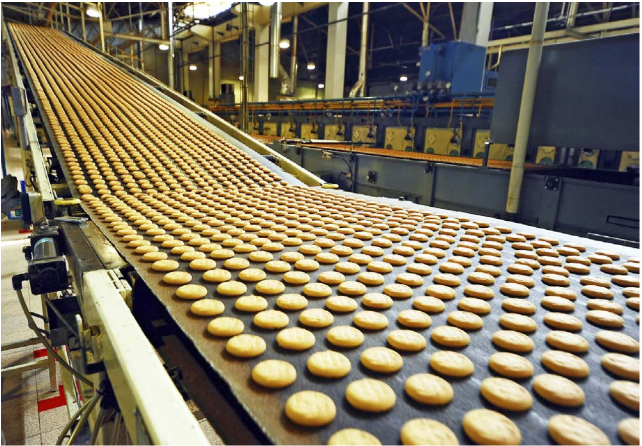
Figure 2.1 The major features of an automated food manufacturing line are high production speed, low unit value, the necessity for cleanliness and product safety. There are very few personnel in the factory. Repetitive inspection tasks, such as this, cannot be performed reliably by human beings for more than a few minutes.
