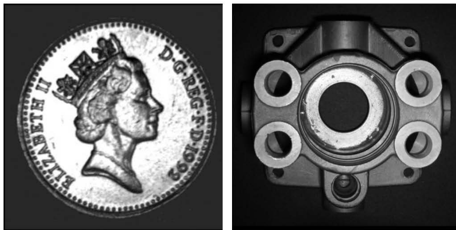
Figure 2.16 Coaxial illumination and viewing. (Top) Optical layout. Unwanted light is indicated by blue arrows. (Bottom-left) Sample image, bright "silver" coin. (Bottom-right) Cast metal component for an hydraulics system. Notice the absence of shadows even in deep crevices. The central feature is a well that is deeper than its diameter.
