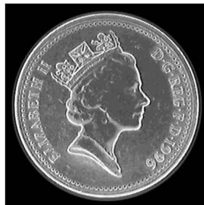
Figure 2.18 Dark field illumination, three variations. (Top) Optical layout for a bottle in fixed position. (Centre-left) Glass vial, illuminated as in [T]. (Centre-right) Aerosol spray cone. Light was projected vertically downwards onto the spray. (Bottom-left) Translucent plastic comb. (Bottom-right) "Silver" coin. Light was projected towards the centre of the coin, at a very low angle, from all directions. This is called Grazing Illumination.
