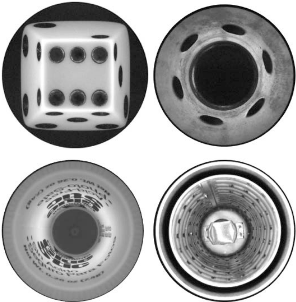
Figure 2.21 Specialist lenses can sometimes make inspection much easier. These images were all obtained using a hypercentric lens. (Top-left) Cube, gaming die. Five of the six faces are visible simultaneously. (Top-right) Internal view of a metal cylinder with six side ports. (Bottom-left) Cylindrical adhesive stick container. Notice that lettering all round the outside surface of the cylinder is visible. (Bottom-right) Internal view of a car oil filter, viewed through a small hole in the top. (These images were kindly supplied by Spencer Luster, Light Works, LLC, Toledo, Ohio, USA.)
