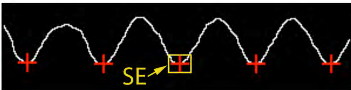
(Row 4) Troughs, found using binary morphology. Structuring element (SE) is defined by that part of the edge inside the yellow box.
